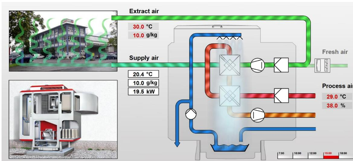
Depending on the cooling demands and outdoor conditions, heat recovery plus evaporative cooling devices can, in non-residential applications, replace significant mechanical cooling provided by chillers. The technology is available but rarely used.
