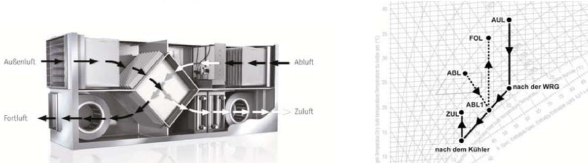
Example: Evaporative cooling using extract air and heat recovery for precooling.
