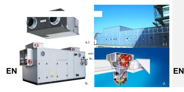
Examples of balanced non-residential ventilation units: a) ceiling mounted balanced unit ( $500-1000 \text{ m}^3/\text{h}$ ) small commercial; b) floor-standing balanced unit ( $5000-12000 \text{ m}^3/\text{h}$ ) medium-size office building; c) extra-large balanced air handling unit (>100 000 m<sup>3</sup>/h); d) rooftop non-ducted balanced unit for warehouses and industry.
